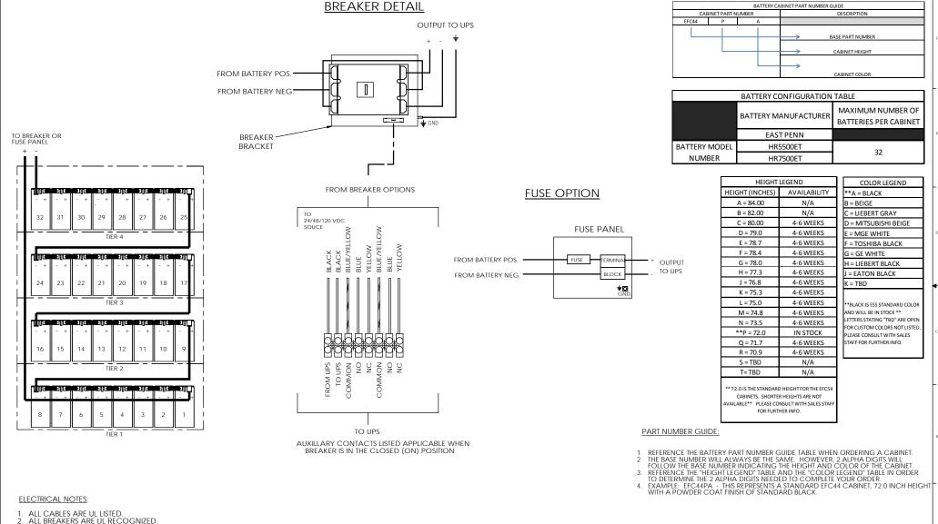
ALL FUSES ARE UL RECOGNIZED, TYPE A50P, A70P OR EQUIVALENT.
